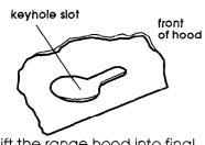
■ Lift the range hood into final position and center. Mark on the underside of cabinet the location of the four keyhole mounting slots. Set range hood aside on a protected surface.
